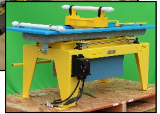
Above, shown with 20 mesh classifier screen & mounted on M5 Stand (optional)
