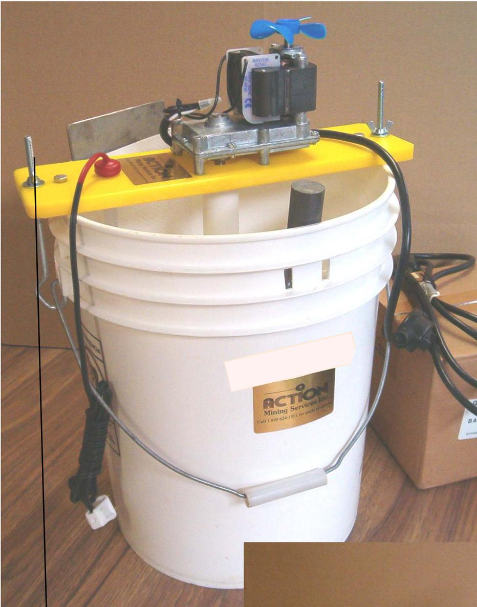
Insert bolts thru holes & tighten wing nuts down on each side to hold motor unit in place. It should be secure enough to keep the unit from moving but not so tight that if the paddle jams in the ore that the motor fan quits turning (the motor will burn out!)
