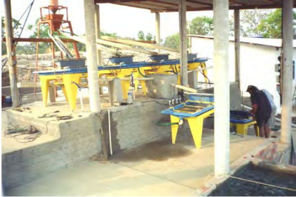
Alternate Production Configuration M7s in production series - final concentration on last M7 table
