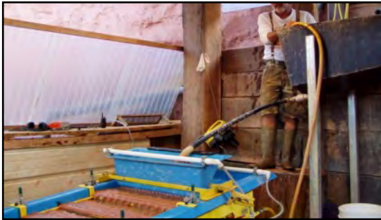
M7 table fed from overhead slurry tank
